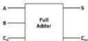
Figure : Block Diagram of a Full Adder
