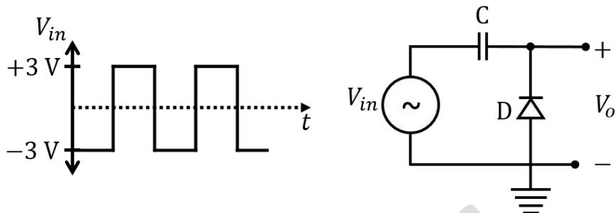
Which one of the following output waveforms ( $V_0$ ) is correct for the given input waveform ( $V_{in}$ )?
