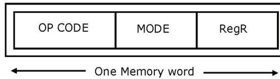
Mode and RegR together specify the operand. RegR specifies a CPU register and Mode specifies an addressing mode. In particular, Mode = 2 specifies that 'the register RegR contains the address of the operand, after fetching the operand, the contents of RegR are incremented by 1'.
